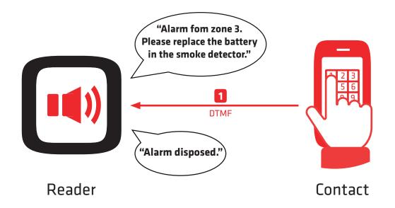
Automated ARC is a module, which - in case of an alarm - automatically calls contacts - one by one.
